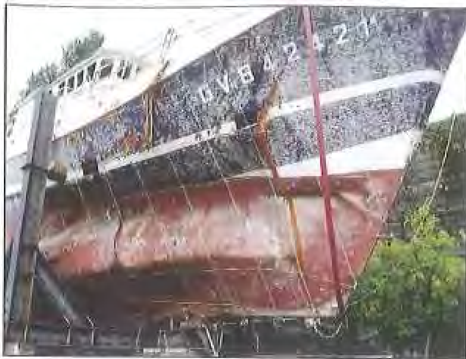
View of the deformation of the starboard side. The photograph shows the deformation in way of the fish hold and the double bottom below it. The bowing of the keel can also be seen.
